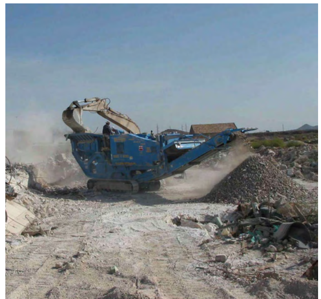
Demolition rubble will be made into aggregate for use as new raw materials.
